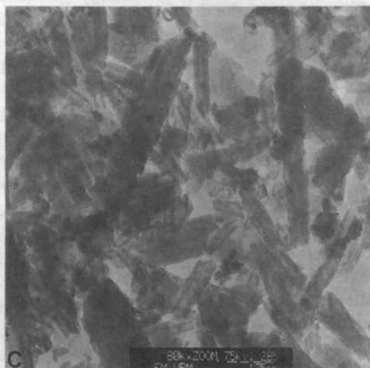
Plate 1C. TEM micrograph of the clay fraction from the A horizon of the Andisol
